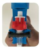
**2b.** After insertion of the TSU release the spring loaded clips to lock in the tube
