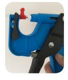
3. You have now completely grabbed the needle. After the needle is inserted into the piston you can release the handles
