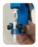
2a. Remove the TSU tube from the pliers by squeezing the two spring loaded clips together, then slide out the tube.
