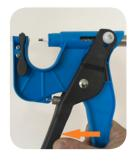
3. Remove the used needle from the pliers by pushing the handles apart. This will loosen the needle and make it easy to remove. You cannot reuse the needle as it has no red plunger.
