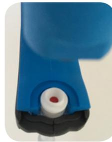
In the used TSU a clear **RED** plunger will be visible indicating the tube already contains a sample and can't be used again.
