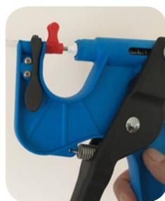
3. You have now completely grabbed the needle. After the needle is inserted into the piston you can release the handles
